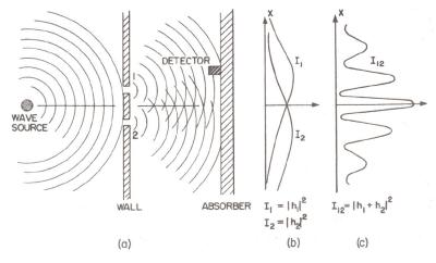
Here the individual results I, and I, for one or the other hole open do not simply add up. The individual wave intensities are the squares of the amplitudes -  $I_1 = |h_1|^2$ ,  $I_2 = |h_2|^2$ . Instead they show the cancellation of crests and troughs that produce constructive and destructive interference. The formula is  $I_{12} = |h_1 + h_2|^2$ . This has the same pattern of bright and dark areas that are found in the "fringes" of light at the sharp edges of an object.
