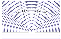
At an angle  $\alpha \approx \lambda/d$ , there is constructive interference (which shows up as the fanning out of light areas in the interfering waves in the illustration). The diagram indicates constructive interference between the 7th and 8th waves from the left and right sides of the slit.
