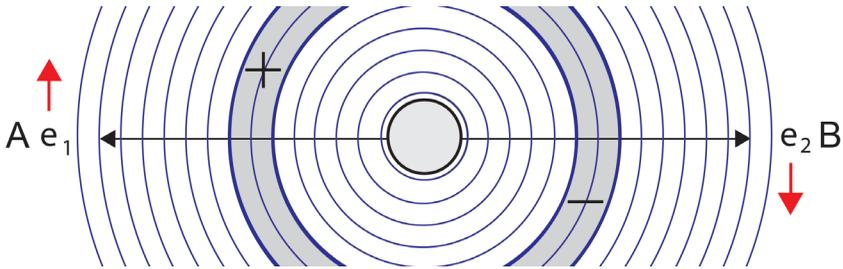
At the start the two electrons are in the same small volume of phase space with their spins opposite, satisfying the Pauli exclusion principle, like the two electrons in the ground state of Helium.
